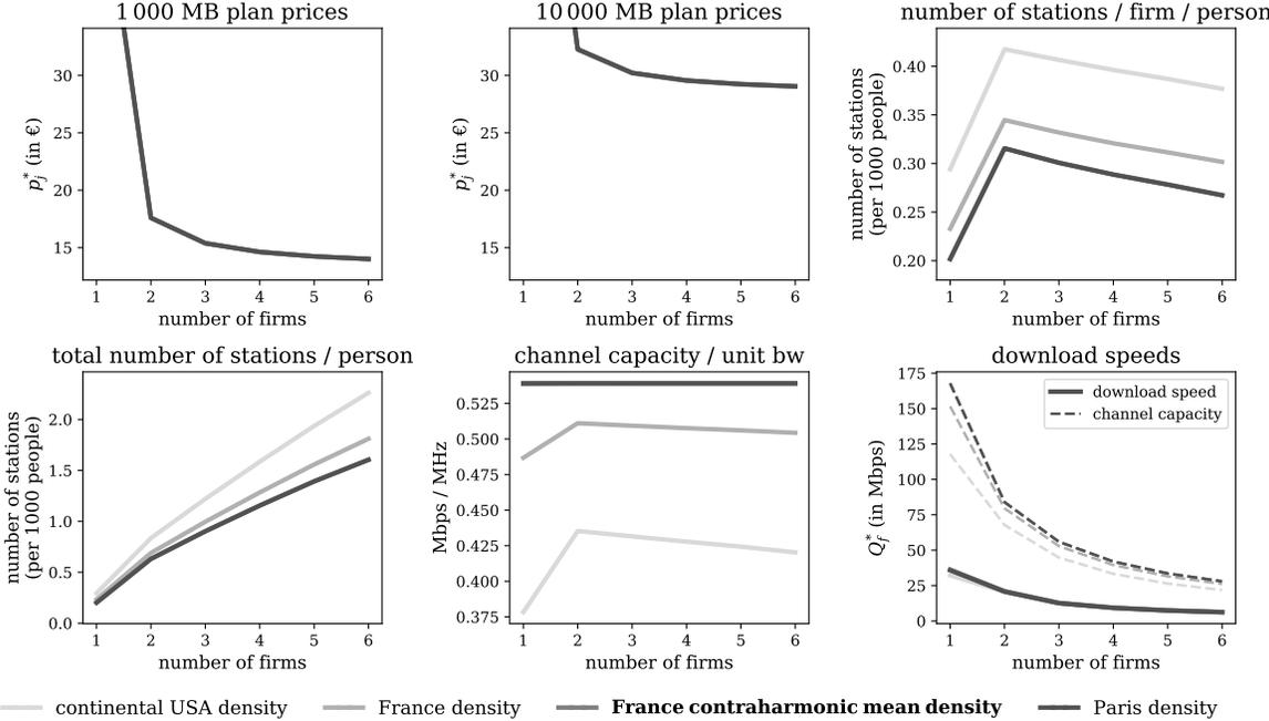
*Note:* Each line in a subplot corresponds to a different population density, with the darker the line, the higher the density. Channel capacity is per base station. Download speeds are the average speed of transmission received by a user, including wait times.
