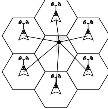
*Note:* The figure depicts the distance between an individual at a random location in the center cell and the base stations that correspond to the six adjacent cells. In determining the channel capacity of the cell, we integrate over the entire area of the center cell, taking into account this interference at each point.
